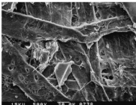
Fig. 4. Scanning electron micrograph of commercial carbon-containing paper.
