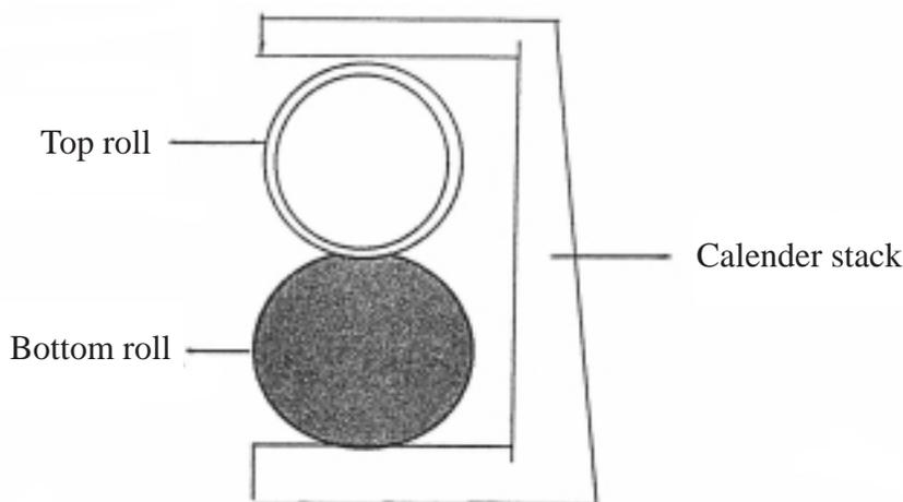
Fig. 1. Top roll and bottom roll of a calender.
