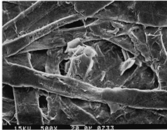
Fig. 5. Scanning electron micrograph of pine carbon-containing paper.
