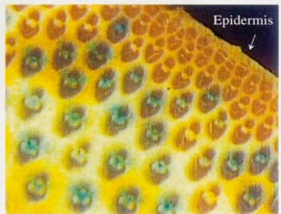
Fig. 3b. Micrograph of colored living Moso bamboo (cross sec. \times 50 ) dyed with basic green dye.
